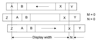
M/N is the number of bits(dots) that parameter 1 (P1) is incremented/decremented by.
