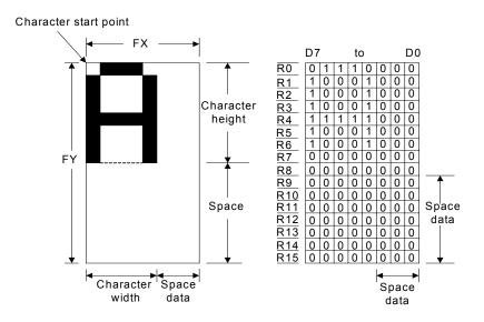
Figure 7-9: Example of Character Display ([FX] ≤ 8) and Generator Bitmap
