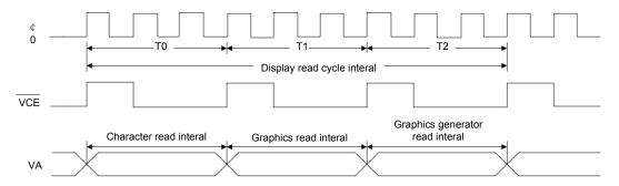
Figure 7-15: Display Memory Basic Read Cycle
