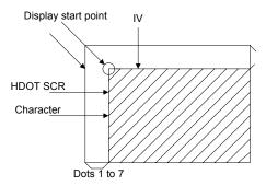
Figure 6-5: IV and HDOT SCR Adjustment
