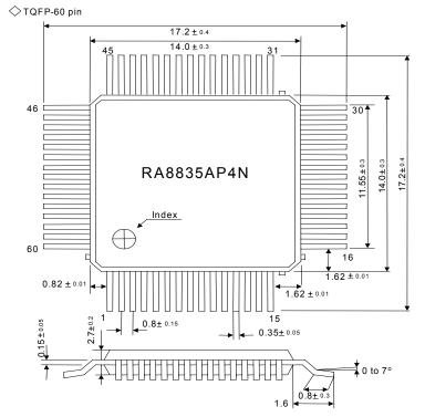
Figure 9-2: RA8835AP4N (Unit: mm)
