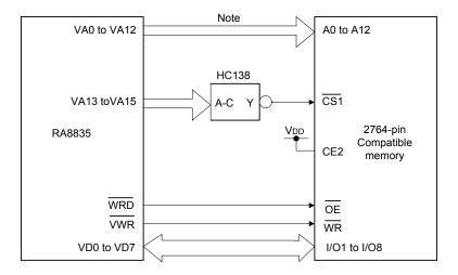
Figure 7-3: Static RAM Interface
