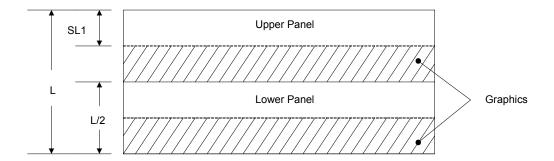
Figure 6-12: Two-panel Display Height
