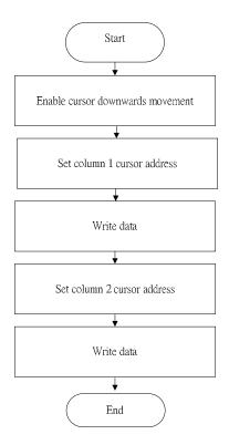
Figure 8-13: 16 x16-dot Display Flowchart
