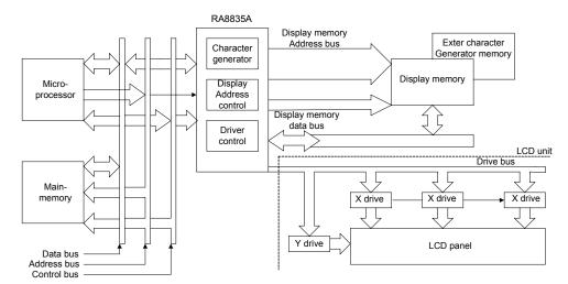
Figure 8-5: System Block Diagram
