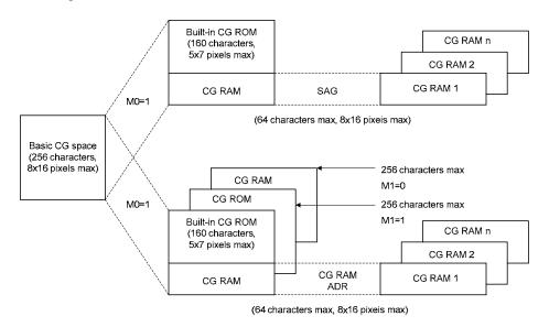
Figure 7-27: Internal and External Character Mapping
