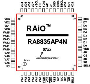
Figure 4-1: RA8835AP3N(QFP-60 Pin)
