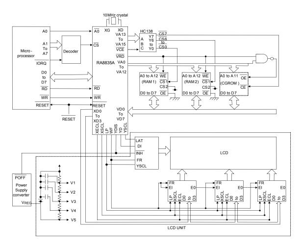
Figure 8-6: System Interconnection Diagram
