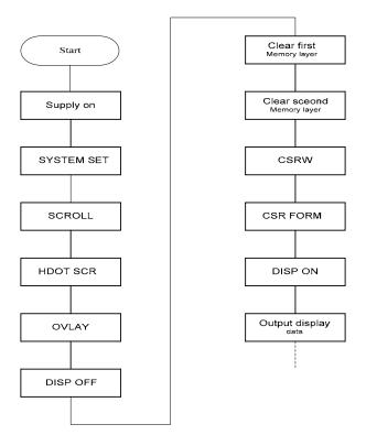
Figure 8-1: Initialization Procedure
