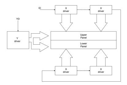
Figure 6-3: Above and Below Two-panel Display
