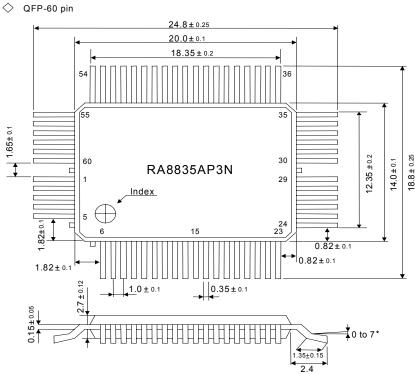
Figure 9-1: RA8835AP3N (Unit: mm)
