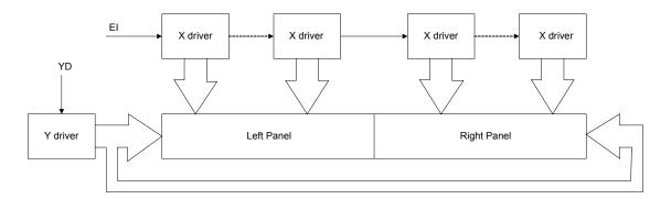
Figure 6-4: Left-and-Right Two-panel Display
