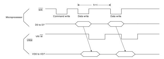
Figure 7-1A: Display Memory Write Cycle
